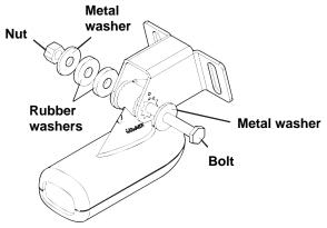
Assemble transducer and bracket.
